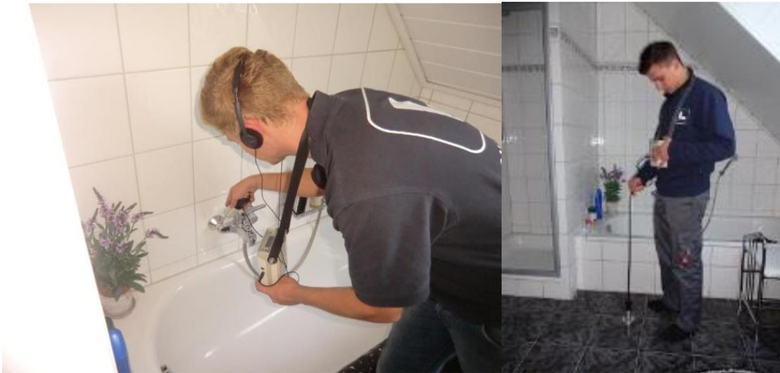
EvaLuate assesses the leak noise at the contact point to the water pipe and tells you where the best grade of the noise is. The closer the distance to the leak, the better the sound (grade) of the leak.
